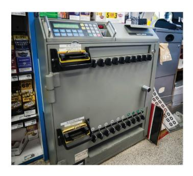
Smart safes are designed to sort and count cash, check for counterfeit currency and automatically communicate the deposit information to the retailer's bank account. The technology removes a lot of the time and effort cash normally requires, with the added benefit that the deposit happens much sooner.
