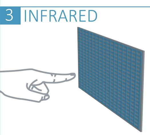
Function: Infrared touch screens rely on light interruption. An array of LEDs and photodetectors create invisible beams of light that when broken activate the touch point.
