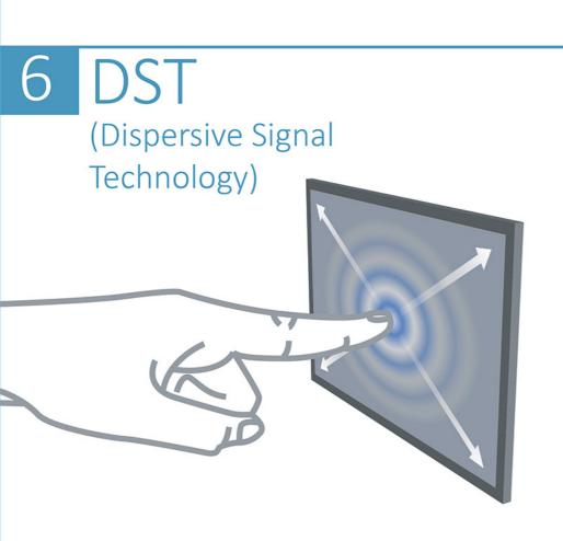
Function: DST uses transducers to detect bending waves (mechanical energy) that are produced when an input device such as a finger or stylus makes contact with the touch surface.
