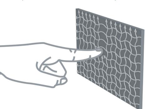
Function: SAW touch screens rely on transducers that emit and receive sound waves. The screen absorbs acoustic energy from the sound wave when it is touched and then records the touch point.
