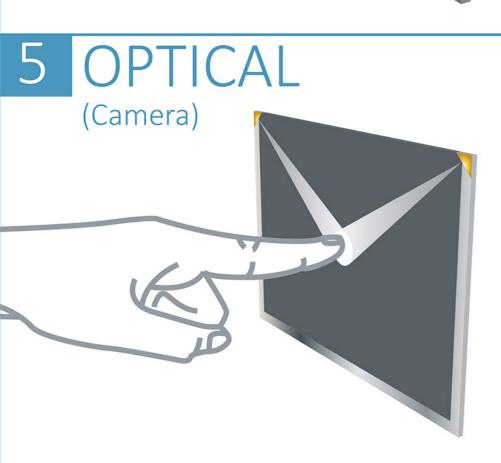
Function: Optical imaging uses sensor cameras that can detect whenever a touch point is made on the screen. This advanced technology allows touch points to be sensed before any physical contact is made.
