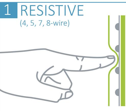
Function: The top layer of the screen touches the lower layer when pressure is applied. This disturbance creates an electrical current identifying the area being touched.
