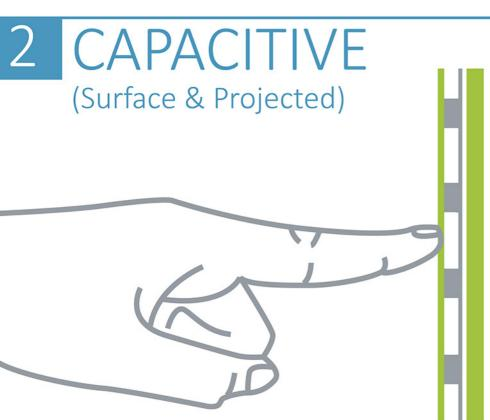
Function: Capacitive screens contain an electrical field that must be interrupted to activate. The screen's electrical field is disturbed by the touch of a finger. The disturbance is measured to accurately determine or track the touch location.
