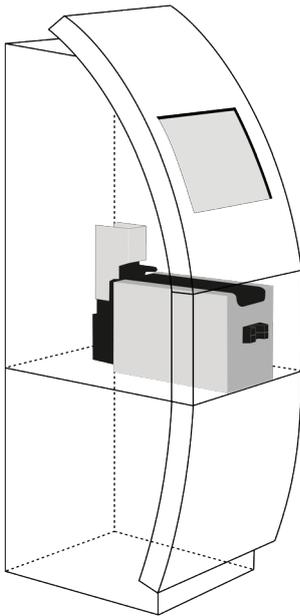
The KM500B and KM2000B printers are distinguished by their high feeder capacity, with 500 and 2,000 cards respectively. Their use, therefore, means limited maintenance of the terminal and avoids frequent reloading of cards and ribbons.
