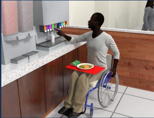
Devices for dispensing food & beverages that are fixed must have compliant operable parts
