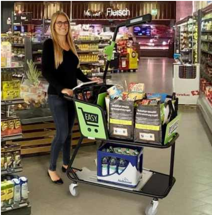
Left: The lateral antenna arm with integrated barcode scanner and control camera is a distinguishing feature of the Easy Shopper
